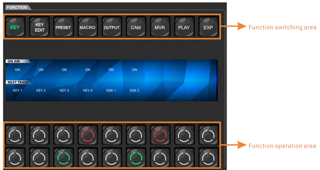
Figure 5-9 Comprehensive control area
