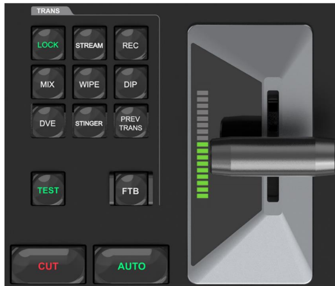
Figure 5-19 Transition control area
