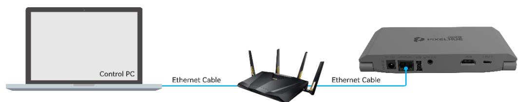
Figure 7-1 Wired LAN connections
