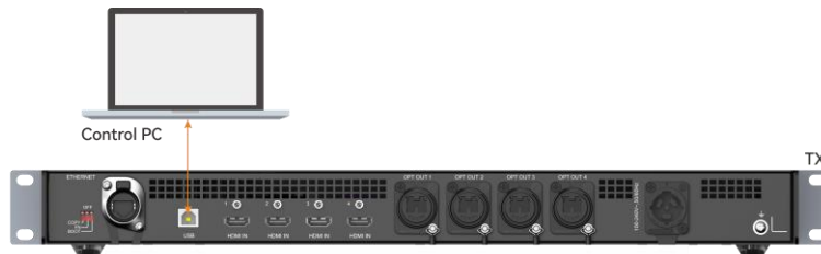
Figure 4-2 TX device connection
